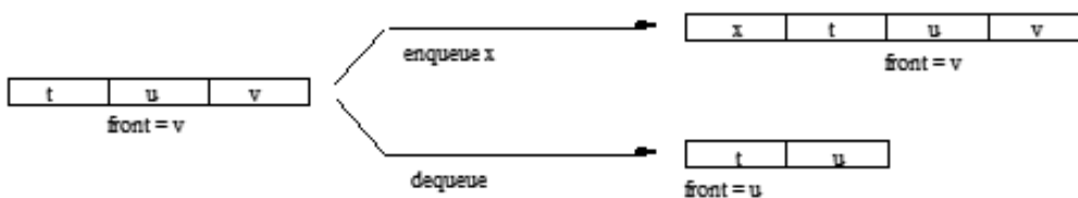
Exhibit 19.2: Elements are inserted at the tail and removed from the head of the fifo queue.
