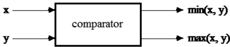
Exhibit 17.14: Building block of sorting networks.
