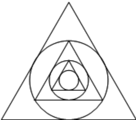
Exhibit 5.10: Interleaved circles and equilateral triangles cause the radius to be exactly halved at each step.
